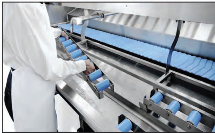
Breakdown area is sloped for better draining of water and debris into the trough. Trough roller assemblies and plate ledges remove easily for cleaning and wipe-down.
