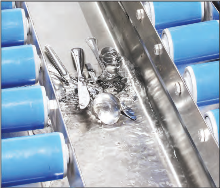
The scrapping table incorporates a magnet to help prevent cutlery from going into the pulper or disposer.
