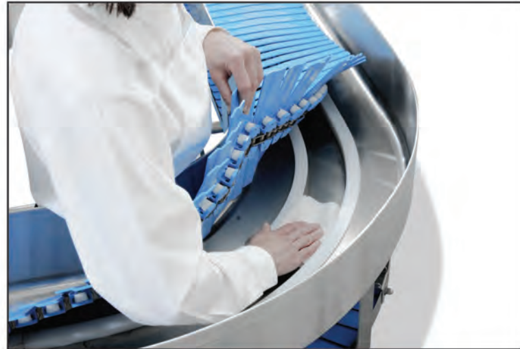
Aerowerks unique slat belt conveyor lifts out easily at any point, even in curves, for simple clean up. The slats are designed with a tapered plane to minimize trapping of food.
