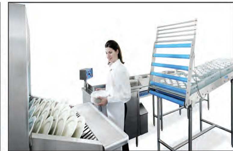
A lift gate on an up-racking system gives the operator maximum control. Lowered, glass/cup racks automatically load into the warewasher. Raised, glass/cup racks accumulate for later loading; or stacked ware arriving on the slat belt conveyor can be manually loaded.
